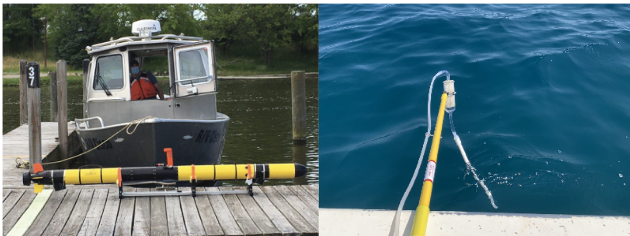
Figure S5.1. Images of sampling equipment used in this study. The autonomous underwater vehicle (AUV) was used to obtain benthic images of Round Gobies (left) and the Smith-Root eDNA Samper fitted with an Envirochek HV filter was used to collect large-volume eDNA samples (right).
